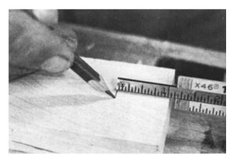
to allow for excess glue. I use a square and a scribe to draw this depth line around all four sides of the tenon board. This marks where the shoulders will go. Don't use a pencil be-
