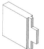
requires extra clamps for gluing the cheeks. But the haunches are necessary to keep the wood from twisting.
