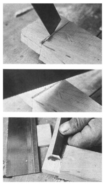
off the tenon corners slightly for easy insertion. Then sand the edge of the tenon so it will fit into the slightly shorter mortise.
