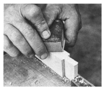
Now finish making your mortise. Take a small chisel and mallet to square off the corners, and a wide chisel (but no mallet) to flatten out the sides. Sand the outside edge of the
