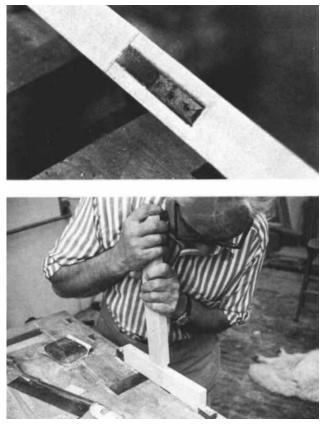
cheeks because that's the easier piece to correct. If the tenon is too loose, you can glue strips of veneer to the cheeks.
