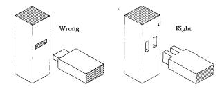
then the cheeks glue into end grain which is not a glue surface. The way to fasten narrow tenons is to use double (or triple) tenons, running the mortises in the direction of the long grain to provide good glue surface. Wedges are used to strengthen the joint. When the tenon is cut to receive the wedge be sure to drill a small hole at the
