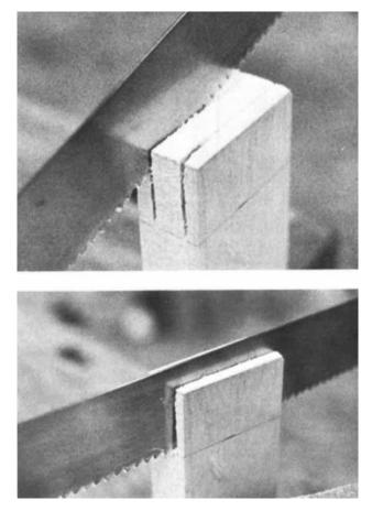
guided at the back by the kerf you made before. You'll also get a little more accuracy in this guiding process if you use a slightly thinner blade for cutting the back lines than you do for cutting the front.
