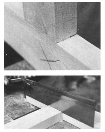
assembled, make a clean saw cut along the shoulder line, making sure not to cut into the mortised piece at all. Do the same for the other shoulder. Don't saw quite completely to the tenon. Instead, finish the cuts with a chisel after the joint is disassembled. If you're making a frame and notice one of
