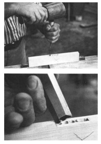
mortise piece as you did the tenon sides and you're ready to try the fit. You should be able to push it in by hand with the weight of your body. If you need to hammer it in, it's too tight and you should shave some material off the tenon
