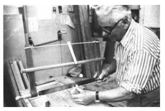
The trick to cutting accurate cheeks is to cut the back line and part of the top first; then turn the board around and cut the rest of the top and the front lines. That way you don't have to worry about following two lines at once. When cutting the front line, the saw blade will be automatically
