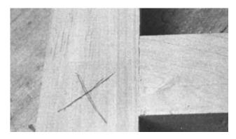
On complicated pieces where the joints may come in at odd angles, I sometimes don't worry about precise fitting of the shoulders during the initial cutting process, but rely instead on the correction cuts to get the fit I want.
