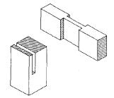
apron is joined to the legs if the table apron is bricklayed round or oval as in a Hepplewhite table. There are several ways to make a mitered mortise and tenon. Often a spline is used, as it is easier to cut. Sometimes
