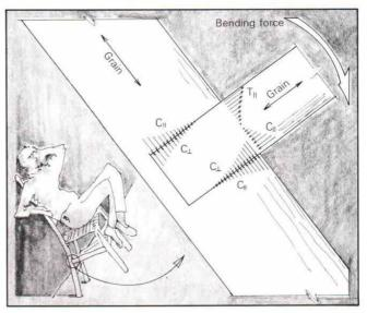
Fig. 1: Tilting, back in a chair racks the joints. The rung tends to bend, causing axial stresses (tension,  $T_{II}$  and compression,  $C_{II}$ ). In turn the rung tenon bears against the mortise walls, compressing the rung perpendicular to the grain ( $C_{II}$ ) and the mortise parallel to the grain ( $C_{II}$ ).
