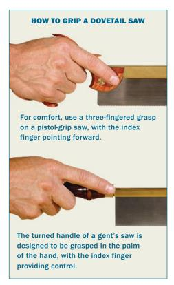
buckling during the cut. The saw back can be made from brass or steel, but a brass back looks good and adds heft, and a heavier saw requires less muscle to use.
