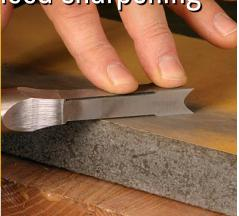
**Smooth the outside surfaces of the chisel.** A chisel with rough outside faces can't be sharpened and won't be easy to plunge and retract. Use fine sandpaper on a flat surface to smooth all four sides.
