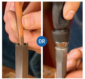
**Hone the bevels.** A little work with a round slip stone (left) or a special, cone-shaped, diamondcoated abrasive (right) produces fresh, sharp edges that ensure a cleaner cut. Use a flat slip stone to remove the burr that results.
