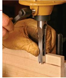
Remove the spacer and raise the chisel until it butts against the bushing. A squaring board ensures that the chisel is square to the fence. Tighten the locking knob.
