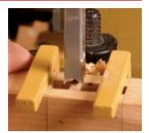
Make two cuts, one at each end of the mortise (left). Then make a series of cuts, leaving a web of wood in between each cut. Last, make cuts (above) to clean out the webs.
