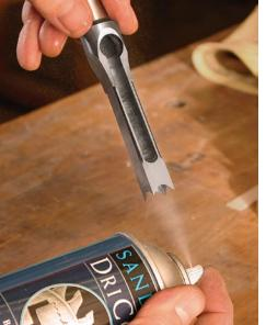
Add some lubricant. To help reduce friction during cuts, spray both the chisel and bit with dry lubricant after sharpening. Later on, when cutting mortises, an occasional squirt of lubricant on the chisel and bit will fight friction.
