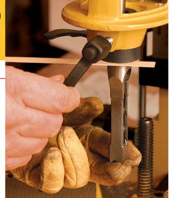
Bit is flush with chisel.
