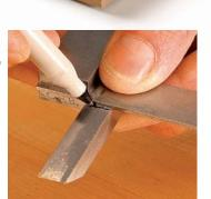
Drive the chisel. Place the tip of the chisel into the cut line on one end of the mortise (bevel facing away from the end), then use a mallet to drive it to the full mortise depth.
