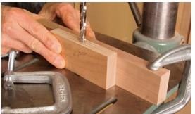
**Drill press does the grunt work.** Use a bit that matches the mortise width. Clamp a fence to the table to ensure that the bit drills into the center of the piece.
