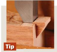
Keep the mortise at least <sup>3</sup>/<sub>4</sub> in. away from the end of the workpiece. Otherwise the endgrain at the end of the mortise could blow out when you drive in the chisel.
