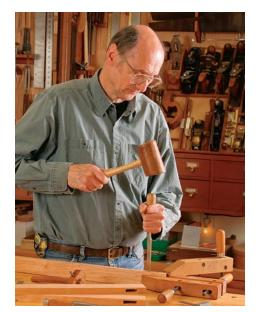
BY CHRISTIAN BECKSVOORT any woodworkers cut mortises by drilling away much of the waste with a drill press, then cleaning up what remains using a bench chisel. The technique is popular because it doesn't require a special machine or jig. It's a challenge, though, mainly because the chiseling process is slow and easily goes awry.
