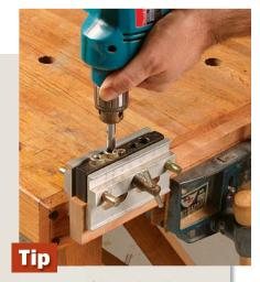
No drill press? Use a doweling jig. It's nearly as fast and just as accurate as a drill press.
