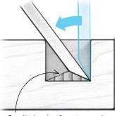
Small triangle of waste remains after levering from both ends.
