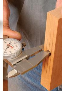
**Dial it in.** After drilling a single hole in the test piece, use a dial caliper to make sure the hole is centered.
