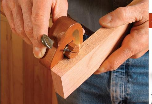
**Scribe the sides.** After marking the location with a pencil, use a marking gauge to scribe each side of the mortise, stopping at the pencil lines.
