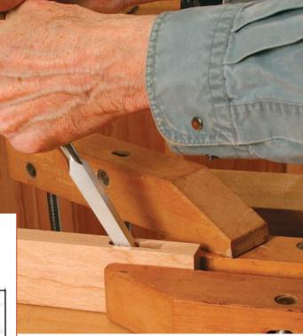
**Lever the chisel.** Lever the chisel toward the opposite end of the mortise. As you do, the square corners of the mortise chisel shave a good part of the waste stock. Repeat from the other end. The levering trick removes all but a small triangle of waste (see drawing, left).
