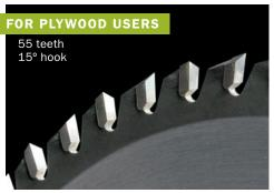
**Plymaster combination blade.** The sequence of 10 ATB teeth and a single FTG tooth leaves clean cuts on plywood, particularly crosscutting.
