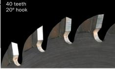
**Cleaner cuts.** Most all-purpose blades have only ATB teeth. A combination-grind blade has one FTG tooth between four ATB teeth, which reduces vibration.
