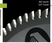
kerf, designed to cut solid wood without tearing out either the top or bottom surface. Because each tooth creates relatively little dust, only small gullets are needed. The hook angle ranges from 5° to 15°.
