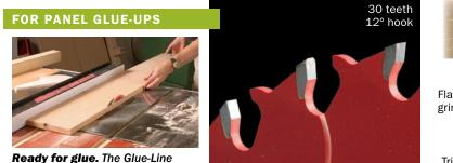
thick. The 30 teeth alternate between FTG and triple-chip grind (TCG).
