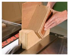
**Good for joinery.** Made for ripping and crosscutting, a blade with a combination grind (ATB and FTG teeth) will leave a kerf with a nearly flat bottom. This is useful for joinery. In this example, it leaves no visible gap between the spline and the box.
