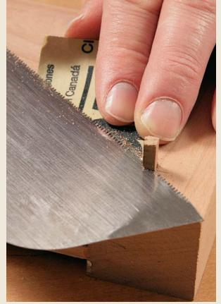
Sandpaper prevents scratches. Where the spine trick won't work, fold a small piece of sandpaper (abrasive side in) and put it under the blade to prevent the teeth from marring the wood.
