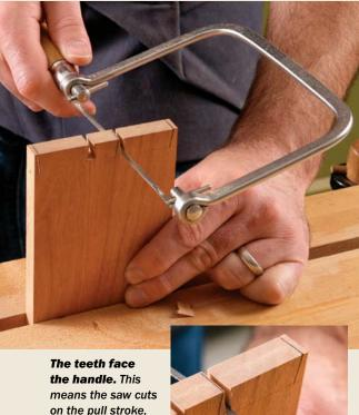
on the pull stroke. which puts the thin, narrow blade under tension so it won't buckle.
