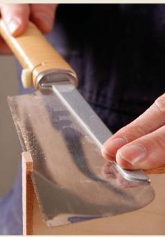
Ride the spine. As you saw, press down on the spine to keep the teeth away from the surface. Use a chisel or block plane to flush the edging.
