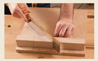
A sawhook is great for small parts. The saw cuts on the push stroke, which helps keep the part against the fence while you cut. A large fence with two kerfs in it—one at 90° (above) and the other at 45° (left)—improves the accuracy of your cuts and prevents tearout. Locate the kerfs so that the fence will support a workpiece on either side of each one.
