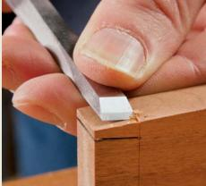
**Cut a clean shoulder.** A crosscut backsaw is perfect for getting rid of the waste in the half sockets on the edges of a tail board. For the best results, chisel an angled groove along the scribed baseline (above) and use the vertical wall of the groove to get the saw started (left). The groove helps to start the saw in a straight cut, so that it naturally cuts down along the baseline, leaving no waste that needs paring.
