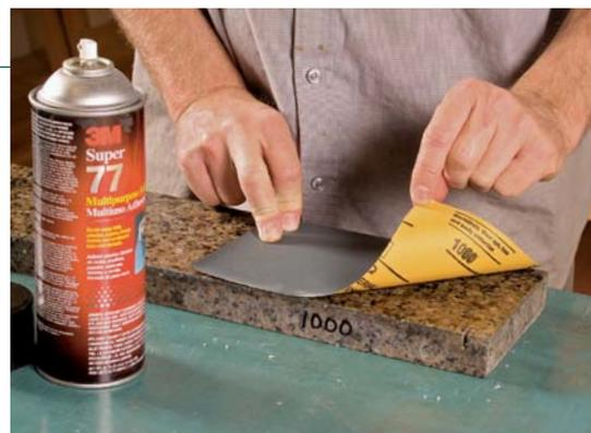
**Easy on.** Use spray glue, which is easy to apply and can be removed easily when it's time to replace the paper.
