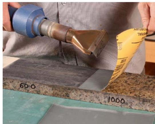
**Easy off.** To pull off the sandpaper cleanly, use a heat gun or hair dryer to soften the adhesive. Mineral spirits cleans up the leftover glue on the granite.
