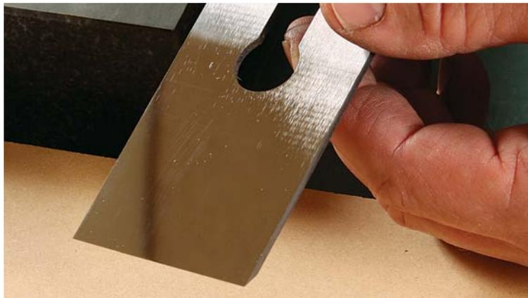
**The payoff.** The back is now ready for work, and you won't need to flatten it again. Removing the burr on the polishing stone (or 2000-grit paper) when you hone the blade is all the maintenance the back needs.
