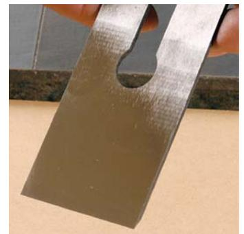
**Work up through the grits.** On the second grit, move the blade in and out until the side-to-side pattern from the previous grit is gone. Then you can move up to the next grit. Continue to alternate between side-to-side and in-and-out movement as you change grits.
