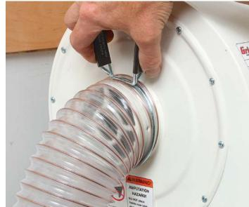
Toolless clamps and fittings. Whether they're spring loaded or the thumbscrew type, they're immediately accessible using only your fingers. The thumbscrew type hold a bit tighter than the spring clamps, but the latter are the fastest to get on and off when switching between tools.
