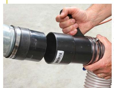
Quick and easy change. Rockler's Dust Right handle and tool ports speed up swapping a 4-in. hose from machine to machine. Once the ports are installed on each machine, the handle slips snugly over the open end, requiring no tools or clamps.
