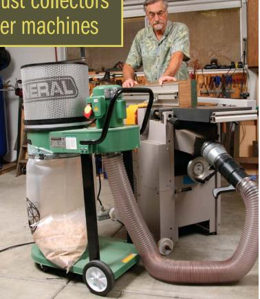
include a jointer and planer. But if your woodworking involves milling rough lumber, a jointer and planer (or a combo machine) are absolutely essential, and so is a dust collector. Jointing and planing wood produces large, heavy sawdust particles, and to move them, a fairly large amount of air volume (about 350 cfm) as well as a 4-in.-dia. hose are required. Shop vacuums aren't suitable for a job that big.
