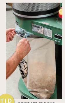
DON'T LET THE BAG GET TOO FULL Empty the bag before it's completely full (shoot for about <sup>1</sup>/<sub>3</sub> from the top of the bag) to prevent clogging and to keep the dust from spilling out during the change-out.
