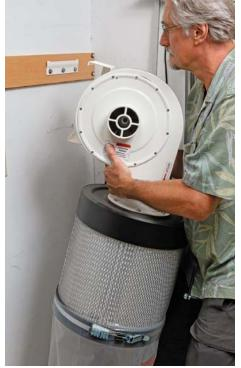
When floor space is tight. Though it can weigh about 65 lb., a wall-mounted dust collector can be moved quickly (it just hangs on a bracket) and stored elsewhere if needed. Get an extra wall bracket or two and move it around the shop where it's needed.
