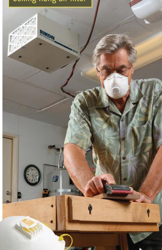
For the dust that remains. Use an airfiltration system. These machines circulate dust particles while they work, so to be really safe, wear a respirator or dust mask when dust is in the air.
