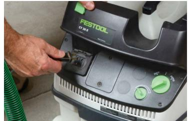
**From a workhorse basic to bells and whistles.** While a sturdy, no-frills model is great to have, a handy feature on higher-priced vacs is the autostart function. When a power tool plugged into the vacuum is turned on, the vacuum starts automatically.
