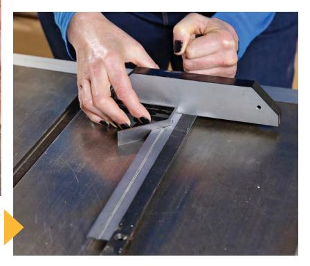
If the slot is parallel to the blade, the tooth will touch the ruler the same amount. If the tooth doesn't touch or it rubs too much, you'll have to adjust the table.
