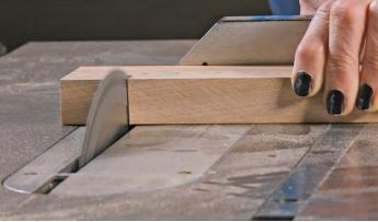
Square the miter gauge. No light should appear between the ruler's edge and the miter gauge's bar while the head of the square is tight to the fence. If it does, loosen the handle and fine-tune the setting.
