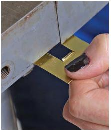
Shim with brass to align the top. To adjust the top, place one or more notched brass shims around the bolts that secure the tabletop to the base. Remember to retighten the bolts afterward.
