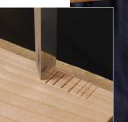
Break up the waste. After laying out the rabbet with a marking gauge, work your way along its length with a chisel, cutting across the grain.
