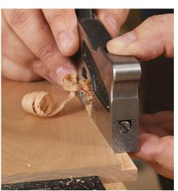
**Finish up square.** As you work down through the rabbet, level out the plane with each stroke until it's cutting a surface square to the shoulder (left). When you've reached full depth, check that the shoulder and cheek are square to one another (below).
