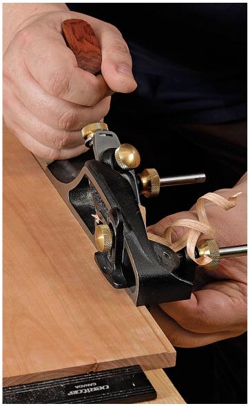
**Start at the end.** Take short strokes at first, starting near the exit end of the workpiece, and taking longer and longer strokes until you are taking full-length shavings. Continue until the depth stop contacts the surface.
