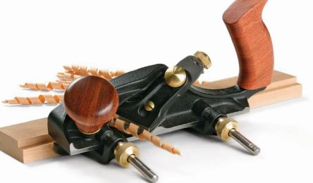
up with a stepped shoulder. One last note: Even though the fence and depth stop control the rabbet's dimensions, I still begin by laying out the joint with a marking gauge. This is helpful when I set the fence and stop, and ensures clean edges along the rabbet.
