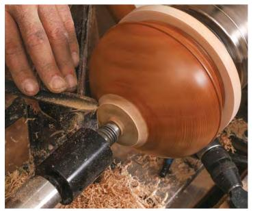
**Transforming the foot.** With the bowl mounted on the jam chuck and the tailstock snugged up for support, transform the dovetailed tenon into a foot with a slightly coved base.
