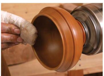
**On with the oil.** Before removing the bowl from the four-jaw chuck, dry-sand the interior and exterior with 220-grit sandpaper, then wet-sand with mineral oil and 320- and 400-grit paper. After that, buff with carnauba wax.
