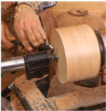
**True up the bowl blank.** Using a bowl gouge with a swept-back grind, first make truing cuts across the cylindrical exterior of the blank, then true up the two flat faces.
