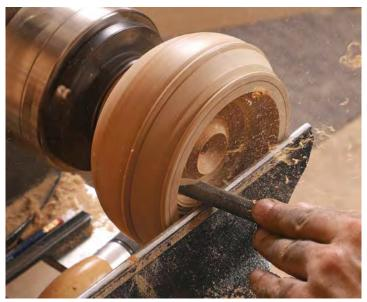
**Excavator.** Begin the rough hollowing at the depth hole and move outward, using a flat-ground deep-fluted gouge. Then, as here, use a swept-back deep-fluted gouge to hollow the incurved area under the rim.
