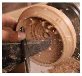
**Finishing up inside.** With the flat-ground deepfluted gouge, take the bowl to final depth and then smooth the walls right down to the bottom.
