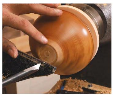
**Fine detail on the foot.** Remove the tailstock and use light pressure with a  $\frac{1}{2}$ -in. shallow detail gouge to embellish the bottom of the bowl with delicate grooves.
