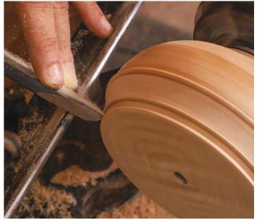
**Shaping the rim bead.** After turning the bead at the rim with a spindle gouge, finalize its surface with a shear scraper.
