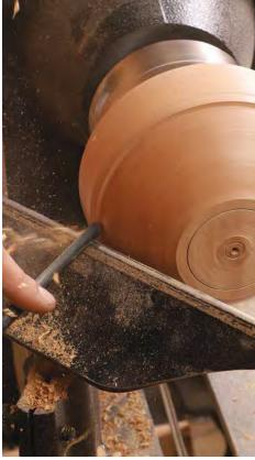
**Shape the exterior.** After some initial rough shaping with a swept-back bowl gouge, refine the exterior shape with a flat-ground bowl gouge.
