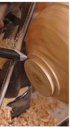
**Tapered tenon.** Once you have refined the exterior curve of the bowl, shape the tenon at the foot, giving it a slight taper.
