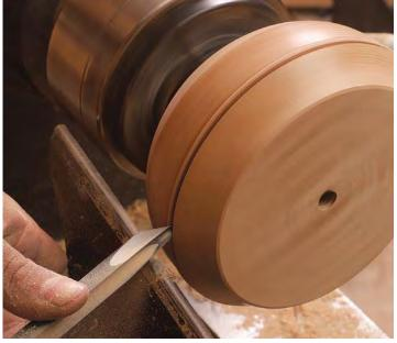
**The bead at the base of the rim.** Having smoothed the outer shape from rim to foot with a spear scraper, use a  $\frac{1}{2}$ -in. shallow detail gouge to form the lower bead.
