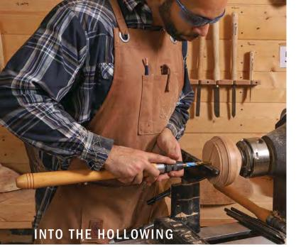
How deep do you go? You can use a twist bit marked with tape to drill a depth hole that will guide the hollowing of the bowl.
