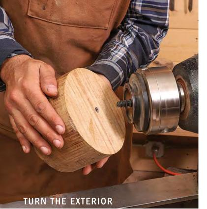
**Threading the blank.** After bandsawing a cylindrical blank and drilling a pilot hole into the center of the top face, mount it on a wormscrew chuck.
