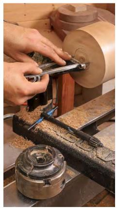
**Sizing the foot.** Before shaping the exterior of the bowl, use calipers to transfer the interior size of a four-jaw chuck to the blank. This will determine the size of the mounting tenon (which will later become the bowl's foot).
