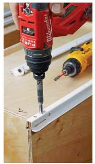
**Drawer side first.** The drawer part of the slide wraps around the bottom of the drawer box and is mounted flush with the box's front edge. Drill pilot holes with a self-centering (Vix style) bit (left) so the slide won't shift when you drive the screws (right).
