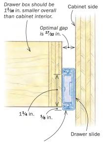
Set the cabinet part of the slide 1/8 in. below the desired position of the drawer box. When attaching the drawer part of the slide, position its top edge 11/4 in. above the bottom of the drawer box.
