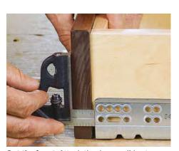
**Set the inset.** Attach the drawer slides to the drawer boxes, and hold the drawer front against the front of the box. Then lock your combo square at the distance between the face of the drawer front and the drawer slide.
