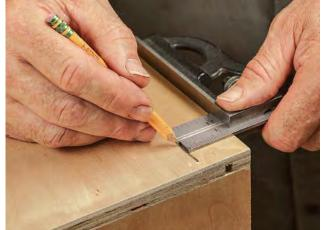
Mark the drawer boxes. If you position the top edge of the drawer section of the slide 1½ in. above the bottom edge of the drawer box, the box will end up in the right spot. Make marks at the front and back of the drawer box.
