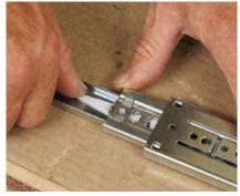
**Pull the slides apart.** Push this small lever to separate the drawer section of the slide from the other two sections.
