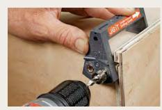
**Drill the drawer back.** Use the guide to drill the two small holes needed at the back of each drawer. (The notches are cut before the drawer is assembled.)
