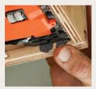
**Up and down.** Small ramps at the front of the slides shift the drawer up and down.
