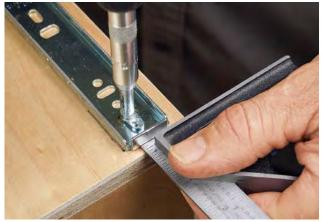
Install the drawer section. Read the instructions to determine the right inset for the front end of the slide, and use a combo square to position it correctly. Again, a self-centering bit ensures that the slide won't shift when you drive the screws.
