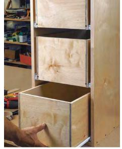
One last check. Once you have installed all three drawers, make sure they are flush with each other when closed. Use the alternate attachment holes to adjust slides fore and aft if necessary.
