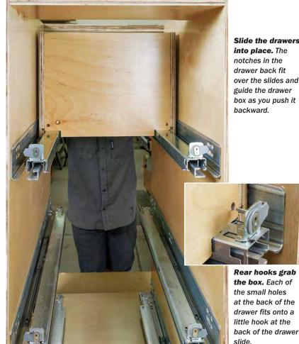
Slide the drawers into place. The notches in the drawer back fit over the slides and guide the drawer box as you push it backward.
